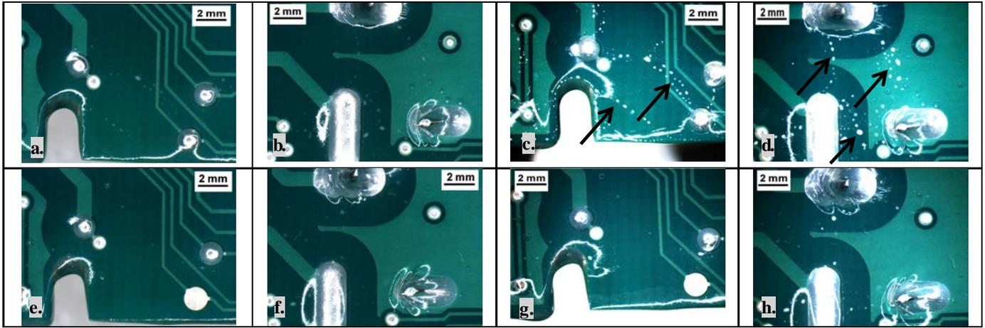
**Figure 8:** Optical microscope pictures of as received wave soldered and coated PCB, a) b) before and c) d) after 3 weeks exposure to saturated humid, and cleaned wave soldered and coated PCB, e) f) before and g) h) after 3 weeks exposure to saturated humid
