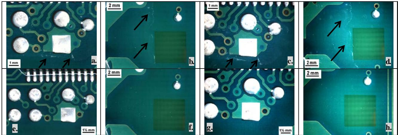
**Figure 9:** Optical microscope pictures of as received selective wave soldered and coated PCB a) b) before and c) d) after 3 weeks exposure to saturated humid, and cleaned selective wave soldered and coated PCB, e) f) before and g) h) after 3 weeks exposure to saturated humid
