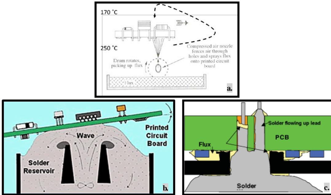
**Figure 2** : Schematics of a) flux spraying at the bottom of the PCB to remove oxide on the through hole component leads and solder pad [10], b) through hole assembled PCB passing through the molten solder wave [11] and c) selective wave soldering process using a pallet [12]
