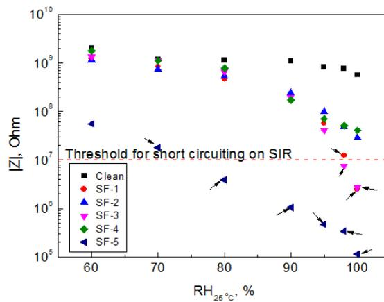
**Figure 4:** Resistance of electrolyte layer between two gold electrodes for different flux
