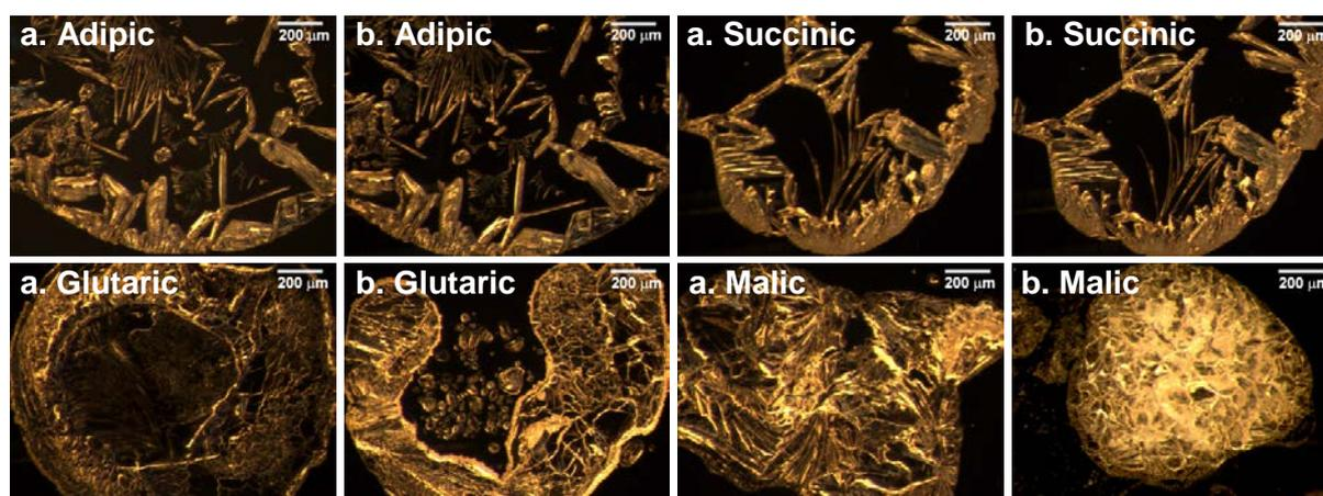
**Figure 1:** The images taken **a.** before and **b.** after the exposure to 98 % RH at 25 °C
