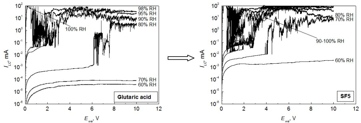
**Figure 2:** Potential sweep leakage current measurement on SIR pattern pre-contaminated with WOA and flux at equivalent concentrations of  $100 \mu\text{g cm}^{-2}$
