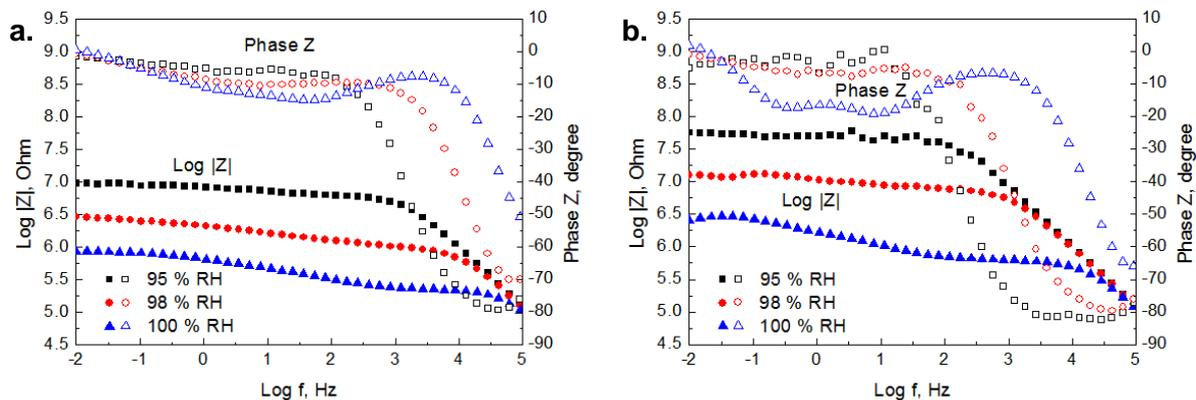
**Figure 3:** Representative Bode plots from impedance measurement between two gold electrodes: **a.** succinic acid; **b.** succinic acid containing flux SF-1
