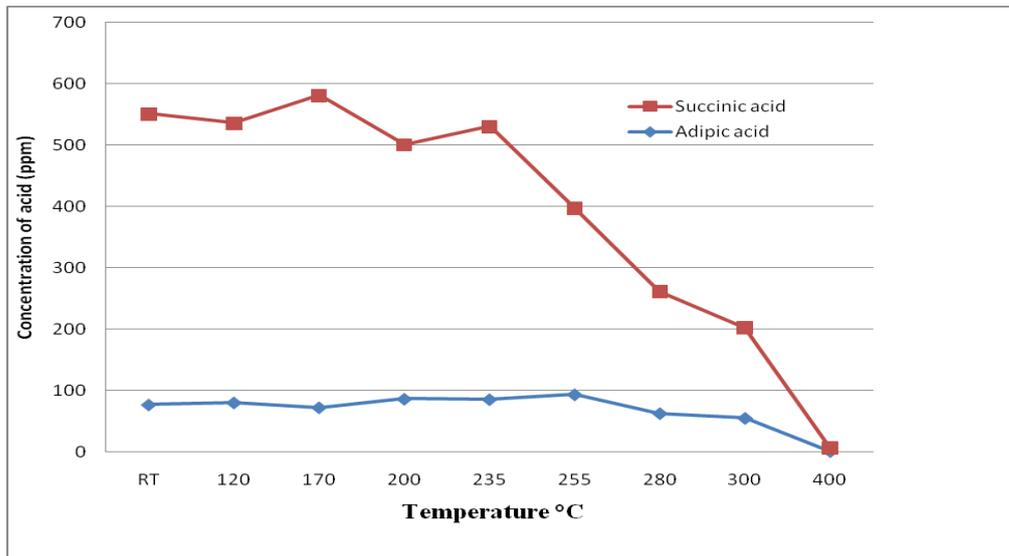
*Figure 6. Percentage of acid component present in the flux as function of deactivation temperature.*
