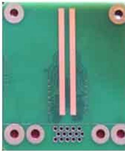
*Figure1. Dual-Copper Electrode system*
