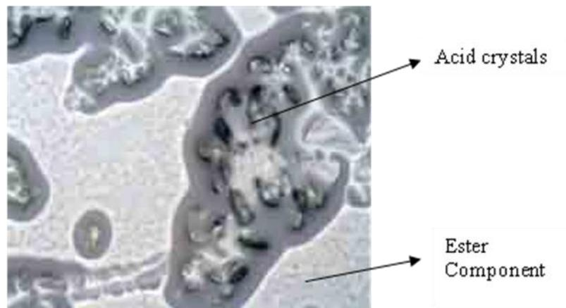
Figure 5. Optical Micrograph of morphology of flux at room temperature.
