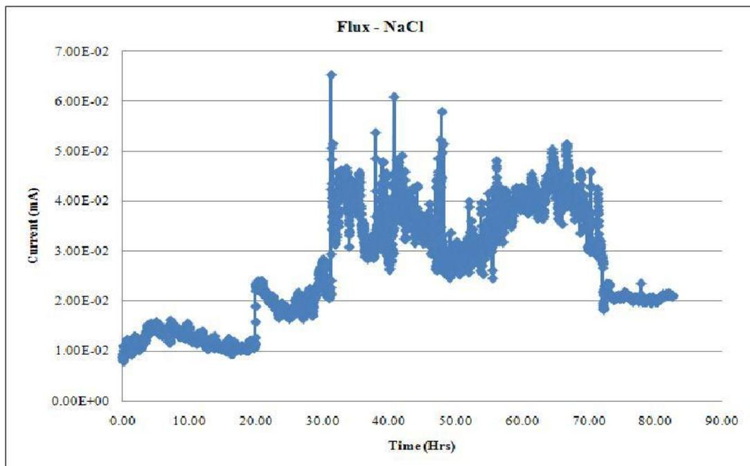
Figure 9(b). Leakage current between the copper electrodes biased with 3V potential, deactivated with flux and coated with the Acrylic conformal coating and immersed in 10 ppm NaCl.
