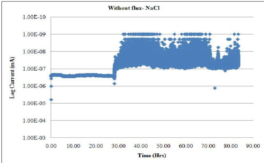
Figure 9(a). Leakage current between the copper electrodes biased with 3V potential and coated with the Acrylic conformal coating and immersed in 10 ppm NaCl.
