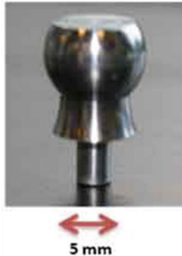
*Figure 3. Dolly used of 5mm diameter*
