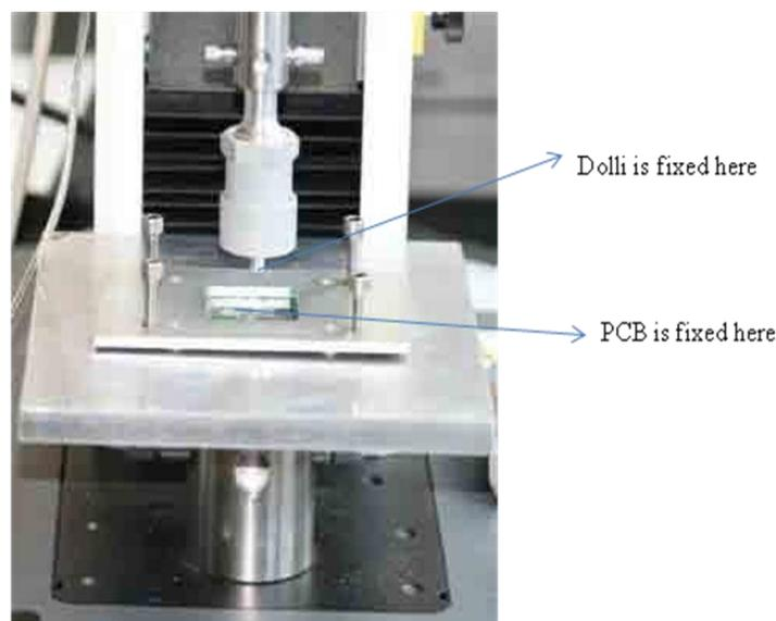
*Figure 2. Fixture for measuring the adhesion strength of the conformal coating on Printed Circuit Board Assembly*
