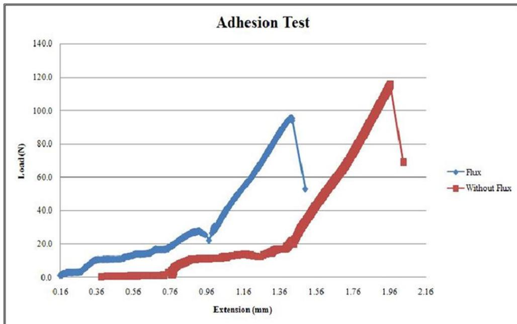
Figure 10. Adhesion strength measurements on Acrylic conformal coating
