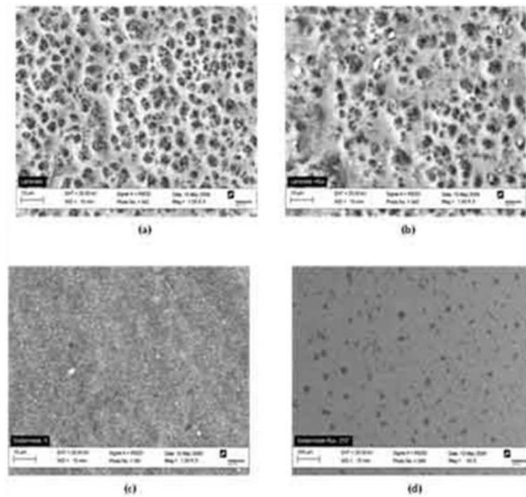
Figure 4. SEM picture of the laminate: (a) FR-4 Laminate, (b) Laminate with flux sprayed, (c) Laminate with solder mask, (d) Laminate with solder mask and flux deactivated at 255°C in oven.
