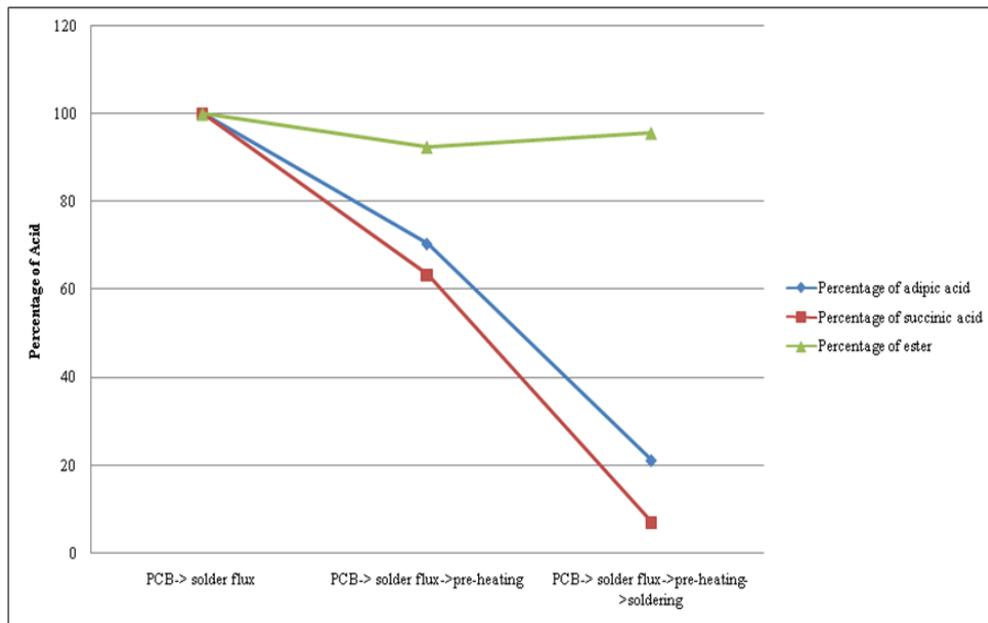
Figure 7. Percentage of flux residue at various stages of wave soldering process
