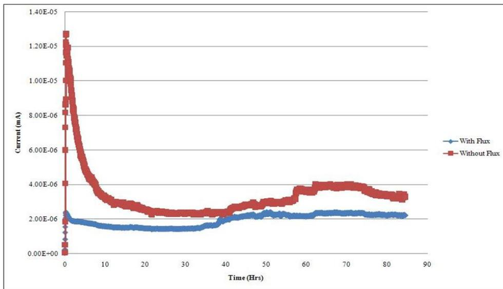
Figure 8. Leakage current between the copper electrodes biased with 3V potential and coated with the Acrylic conformal coating and exposed to 60°C and 96 %Humidity.
