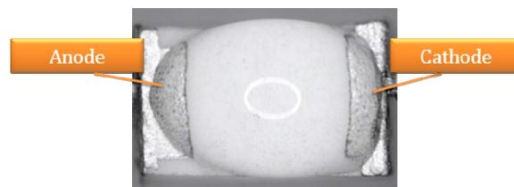
Figure 4: CCR with water droplet added for simulating local condensation. When potential bias is applied, one terminal will act as cathode, while the other will act as anode.
