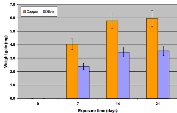
Figure 10. Weight gain of copper and silver due to corrosion in the Battelle test. Copper: orange/left, silver: blue/right.
