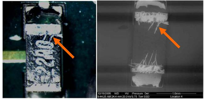
Figure 3. Sulphur attacks on a chip resistor. The ‘needles’ consist of  $Ag_2S$ . Seen both in lab tests and from the market. The resistor is still functioning.
