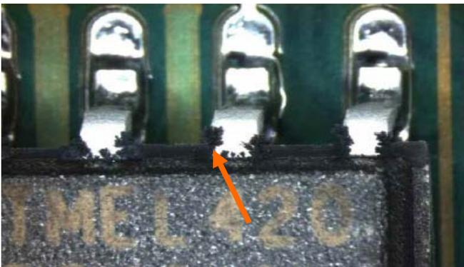
Figure 2. Sulphur attacks on IC [d] leads. The black deposit consists of copper and sulphur. Seen both in lab tests and from the market. The IC is still functioning. [4]
