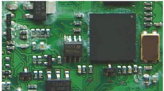
Figure 4. White residues, visible after being exposed to high humidity at a customer. The PCBA has failed.
