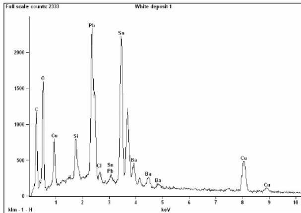
Figure 6. SEM-EDX spectra from the areas with white flux residues as seen in Figure 4.
