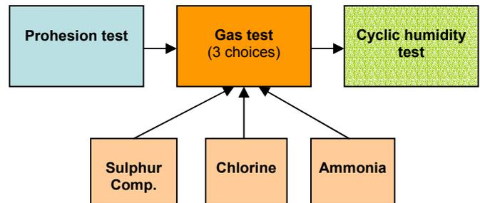
Figure 7. Flow diagram of the ‘Aggressive sub 3 test’.
