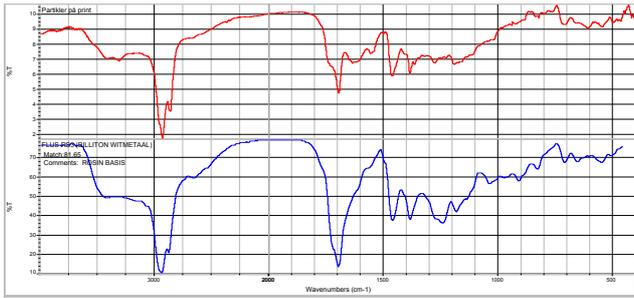
Figure 5. IR-spectra of white residues from a PCBA (upper red curve) and the applied flux (lower blue curve).
