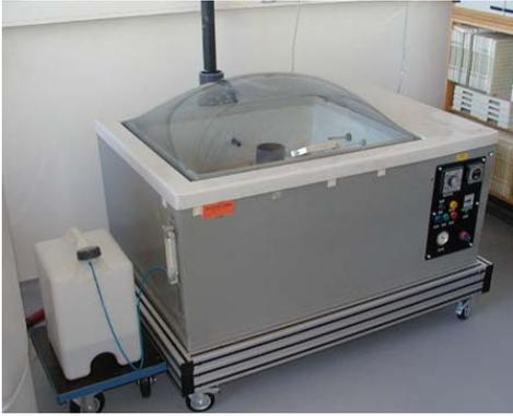
Figure 8. Prohesion chamber used at Danfoss.
